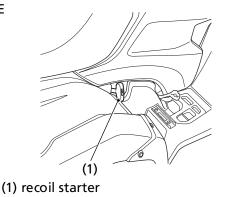
The recoil starter (1) is used to start the engine when the battery is low. See Using the Recoil Starter (Canada only), page 86.
