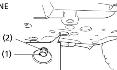
(1) engine oil drain bolt
