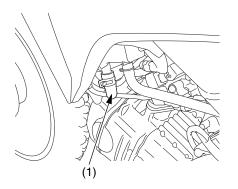
• Drain the deposits into a suitable container by pinching the crankcase breather tube (1).
