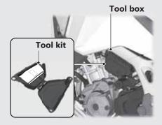
Removing the tool box P.257
