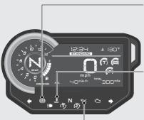
(S) ABS (Anti-lock Brake System) indicator Comes on when the ignition switch is turned to the ON position. Goes off when your speed reaches approximately 6 mph (10 km/h).
