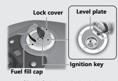
Do not fill with fuel above the level plate. **Fuel type:** Unleaded gasoline only **Recommended fuel octane number:**Pump Octane Number (PON) 86 or higher. **Tank capacity:** 4.28 US gal (16.2 L)
