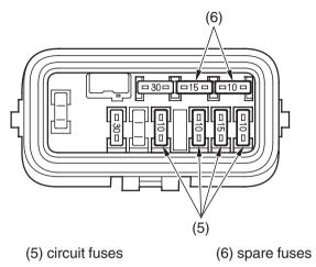
6. To check or replace a circuit fuse (5), pull the old fuse out of its retaining clips.
