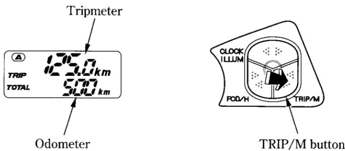
The tripmeter will show mileage in two sub modes, "tripmeter A" and "tripmeter B."
