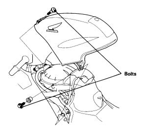
Front Lower Cover Remove the bolts then slide the cover forward.
