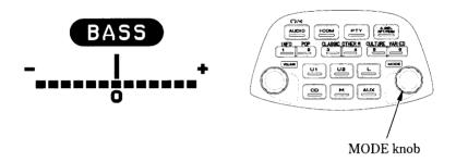
To select the Treble control, push the MODE knob two times, and "TREBLE" will appear on the display. Then, within five seconds, change the treble control.
