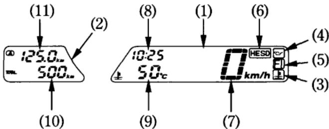
Odometer/Tripmeter display (2) includes the following functions:
